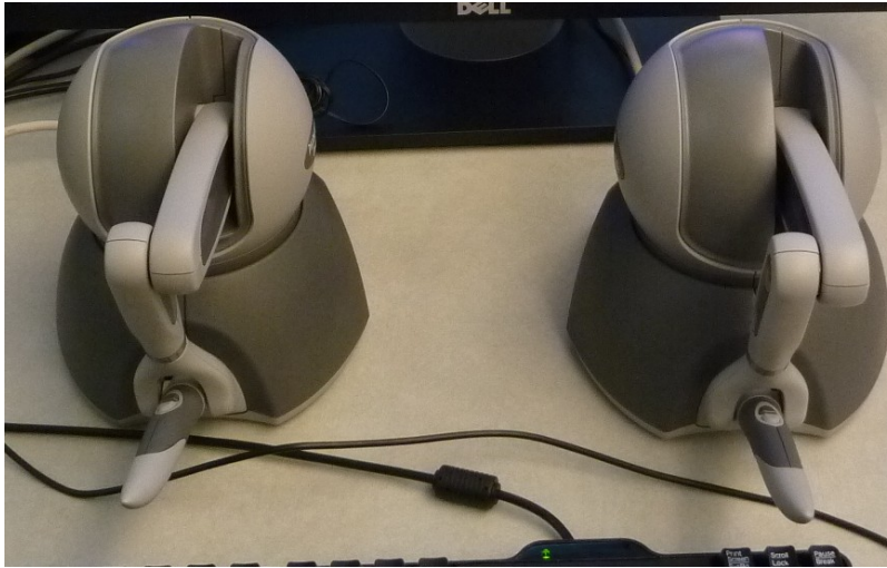
The SensAble Phantom Omni haptic devices
